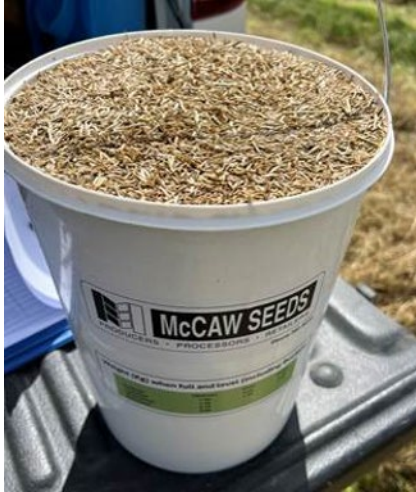
Figure 3. Bucket used to test the hectoliter weight and quality of the harvester grain tank sample. The bucket weighed 1.9kg (minimum weight for bucket according to John's label = minimum weight 1.9kg, good ryegrass weight 2.00kg and heavy 2.1kg)
