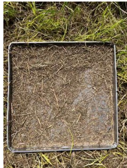
Figure 2. Drop pan with offal and seed in it, assessed losses were: 200kg/ha, 8.3% loss on 2400kg/ha crop.
