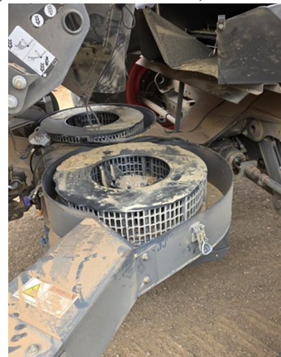
Seed destructor mounted on a Claas Lexion combine, Corowa Seeds, VIC
